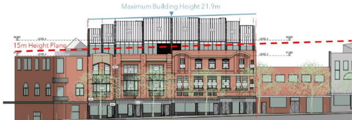
Figure 19: Elevation of Group 3 with the 15m Sydney LEP 2012 height control as viewed from Oxford Street
