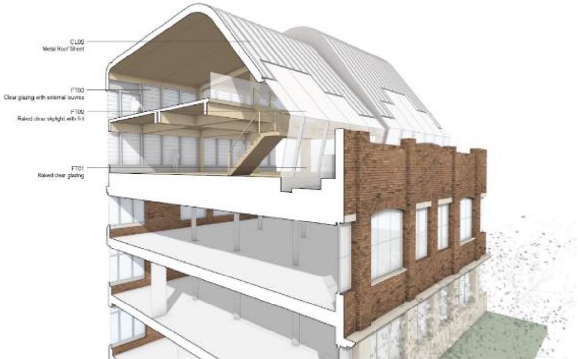
Figure 24: Section through Group 1
